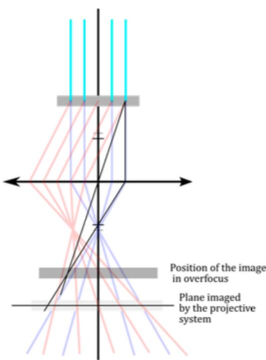
The final step requires to draw the diffracted and undiffracted rays in this new configuration. On the plane imaged by the projector system, diffracted and undiffracted rays coming from the same place of the specimen do not converge at the same place. The diffracted beam forms an image slightly displaced (to the right on the drawing). This explains the ghost image, which is then obtained from the diffracted rays, and is hence a bright and displaced image of the specimen.
