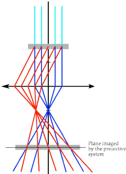
The next step is to draw the image formation in overfocus. The objective lens has a stronger excitation. The focal points move closer to the lens. With this information, we can find the plane where the image is now forming.
